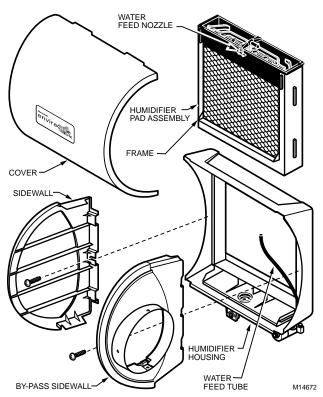
Fig. 5. Location of humidifier parts.
